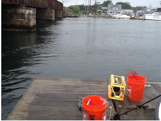
Caption: FSI's ACM being deployed from Eastwinds Lobster and Grill dock in Buzzards Bay, MA. Buckets contain computers and wifi devices for data transmission.
